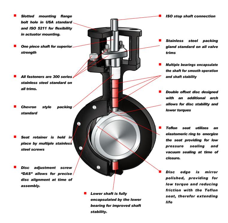
Flow Line Series 76/77 valves are also offered 30"-60" in diameter for ANSI class 150 in wafer, lug, and flanged end.
