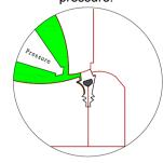
Disc in closed position; line pressure applied from the bottom
