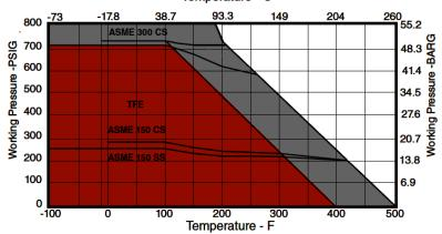
*Note*: TFE and RTFE seated valves are rated to 55 psi saturated steam.
